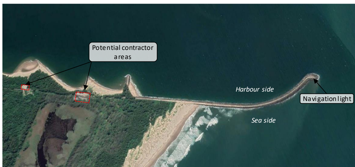
Figure 2.2.1-1: South Breakwater layout.
